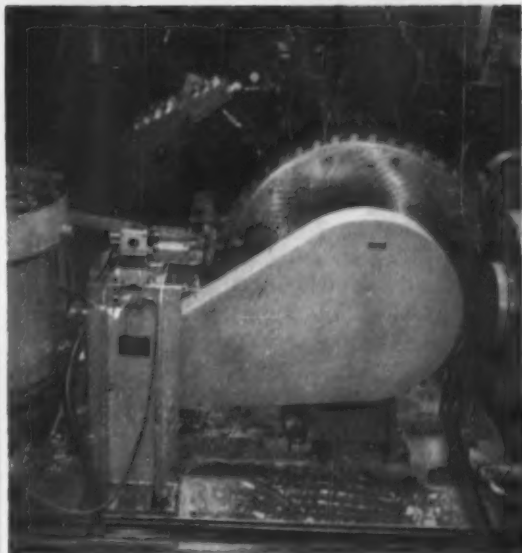
Top—Left: Fig. 2—Parts segregated for undersize holes are brought within limits on this honing setup.
